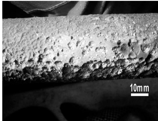
Metal dusting in a drain line of a Ni based alloy located in a steam superheater Example of pit formation
