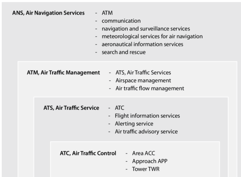
Figure C.1: The ANS system and its components according to ICAO. 14
