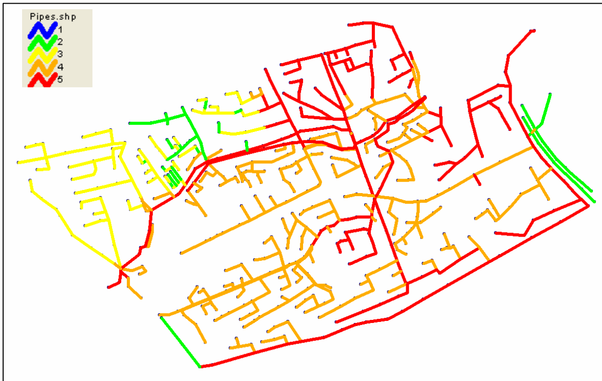
Figure 9: Pipe condition classes at 2050 (CC1 corresponds to excellent condition; CC5 to failing pipes)
