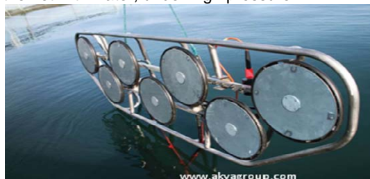
Cleaner discs utilized for high pressure cleaning of net pens. Cleaner discs are guided up and down along the net side, and flush away the biofouling under high pressure Photo: AKVAgrou ASA).
