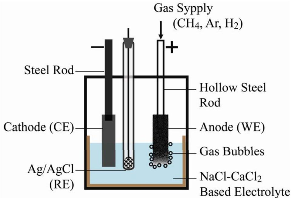
*Experimental setup for electrochemical measurements*
