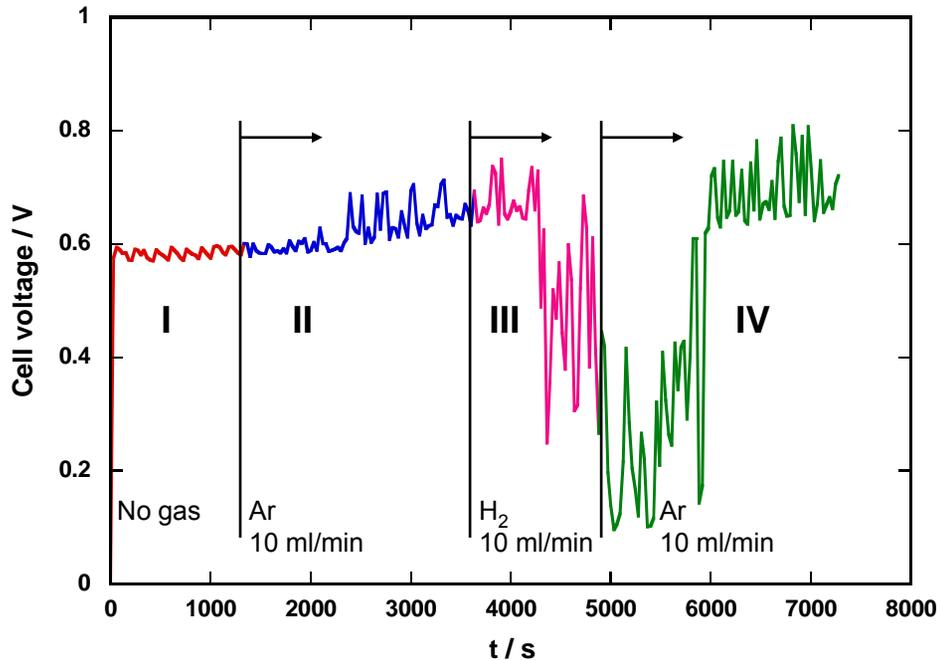
**Electrolysis with constant current 0.1A in CaCl<sub>2</sub>-NaCl(70-30 mol %)-CaO(16 mol %)-AgCl (4.7 mol %) melt; current density, 30mA cm<sup>2</sup>**
