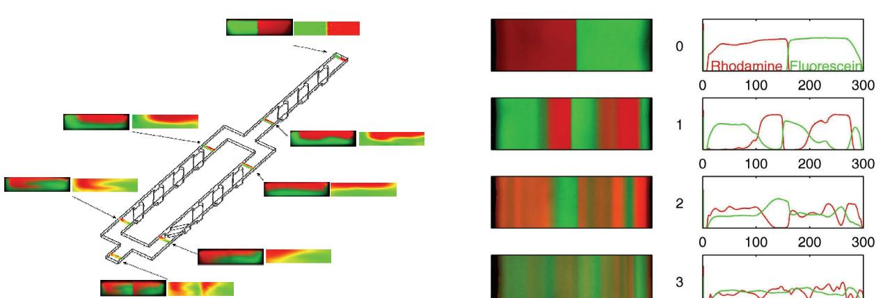
Fig. 3: Simulated and measured concentration distributions within one mixing module
