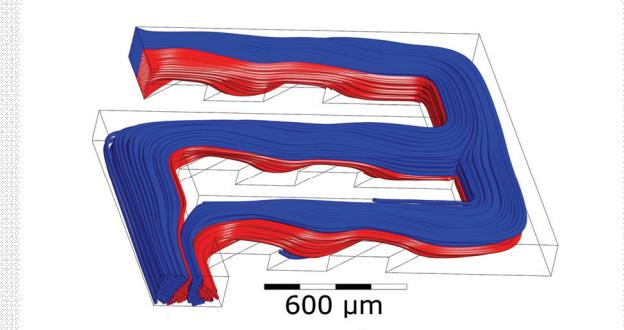
Fig. 1: Simulated flow field in one compact mixing module showing lamination
