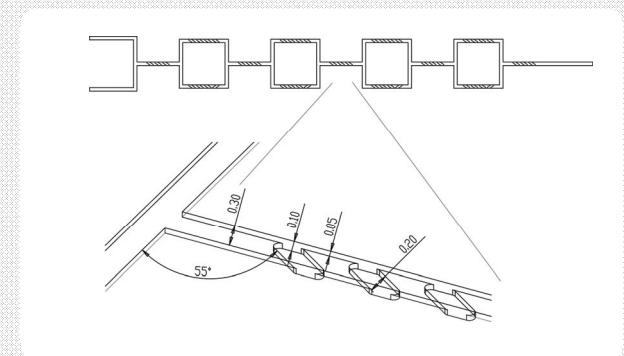
Fig. 2: Above: Design showing four mixing modules.
