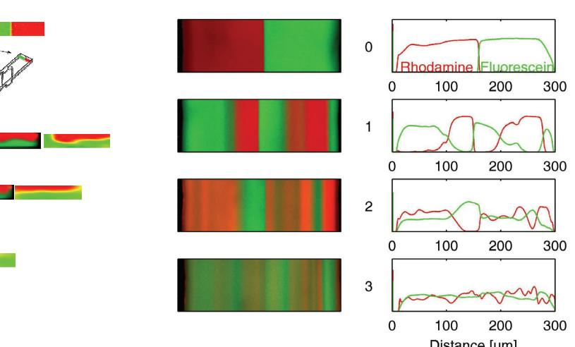
Fig. 4 Left: Confocal microscopy images showing planes at  $z = h/2$ , where  $h$  is the channel depth. The images show the intensity after 0, 1, 2 and 3 full modules.
