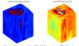
$85\times85\times8$  cells, 55.192 active, 75 blocks pressure boundary conditions
