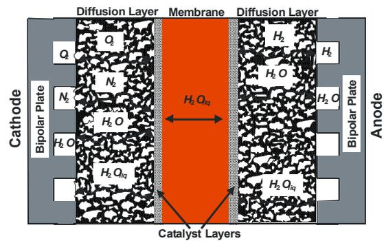
Fig. 1: 1-D Model of the HT-PEFC
