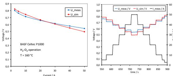
Fig. 3: Verification of Simulation Model: a) I-V curve and b) I,V –steps on load change of Celtec P 1000-MEA.
