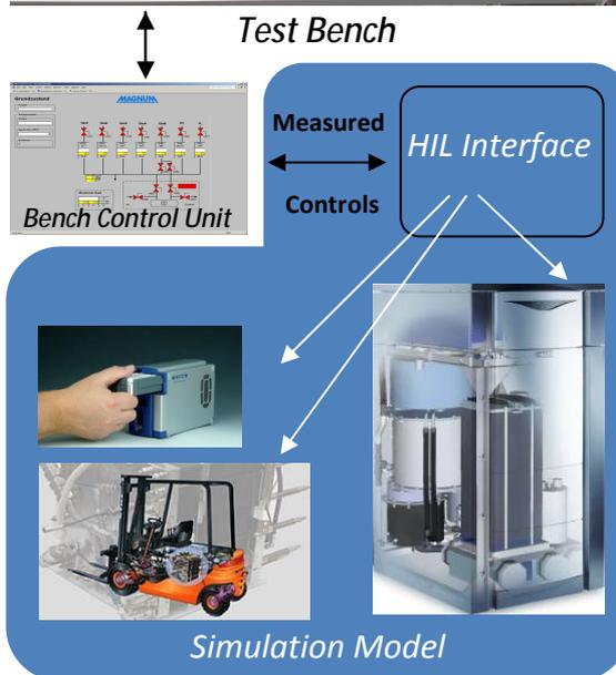
Fig. 2: HIL- Set up for Fuel Cells
