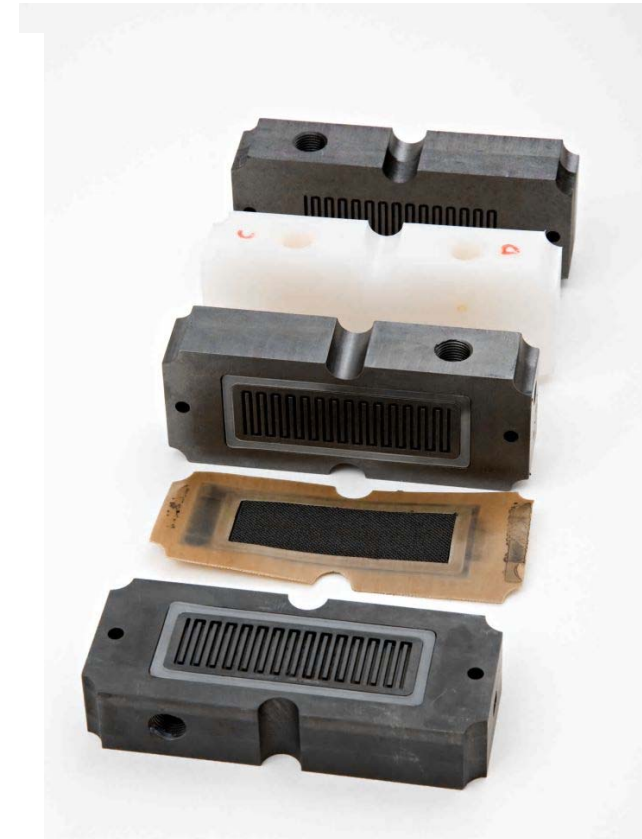
Figure 11 Cell design for stainless steel and coating testing
