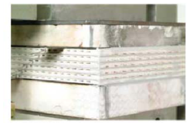
Figure 3. A 5-cell cross flow stack assembled from co-fired cells and interconnects. The air and fuel channels are seen on the two faces of the stack shown.
