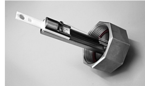
Langasite resonators in alumina sample holder of gas reformer sensor
