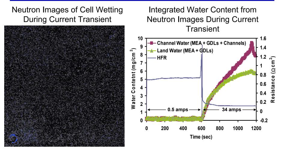
Minimum flows at 82cc/min and 333cc/min at the anode and cathode @ 0.5A. At 34A it is 1.2 and 2.0 stoich flows.
