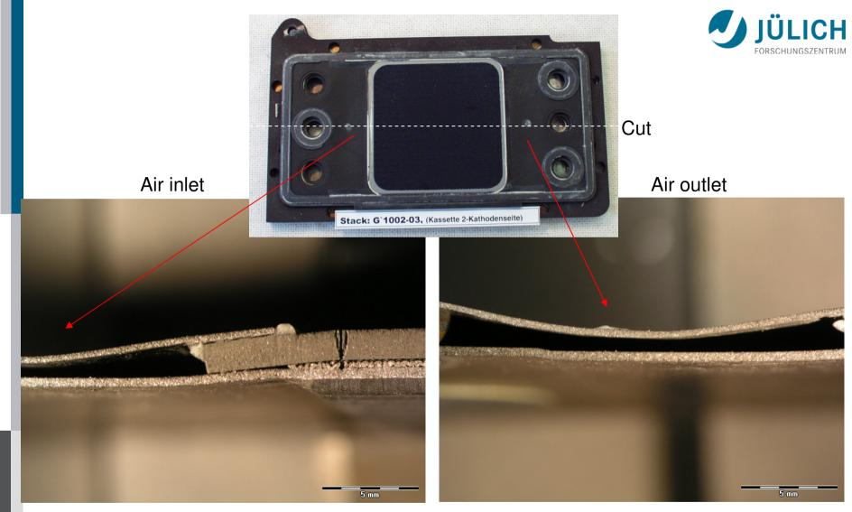
Large manifold made from thin metal sheets is not geometrically stable at high temperatures Results are short circuit or cell fracture
