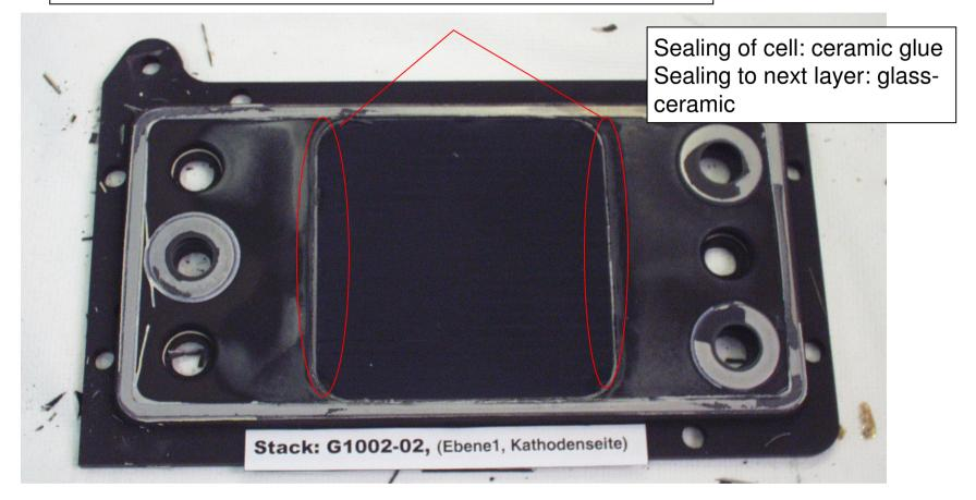
Before further dismantling took place the origin of the short circuiting was investigated using infrared camera imaging (thermography).
