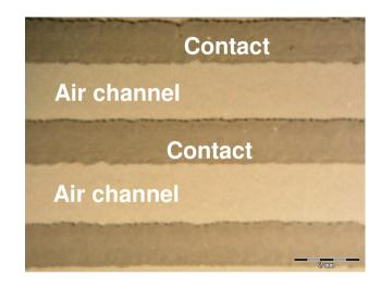
Small contact width compared to standard design
