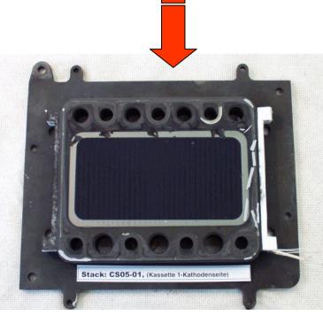
Using a combination of metallic and glass-ceramic sealants.
