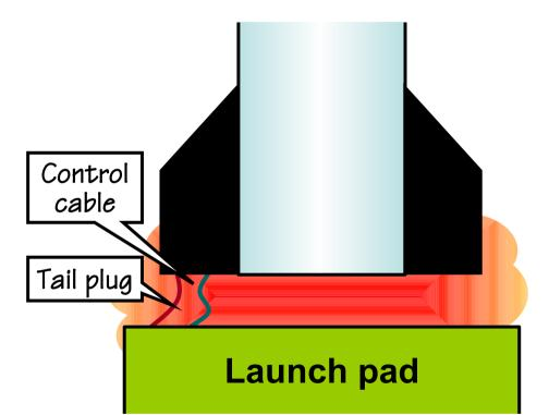
This condition created a sneak circuit, defined as an unintended current path, which causes an unwanted function to occur or which inhibits a wanted function.
