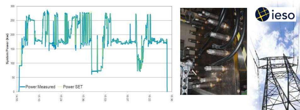
HySTAT<sup>™</sup> electrolyzer provided frequency regulation by responding to real-time frequency regulation signals from the IESO on a second-by-second basis.
