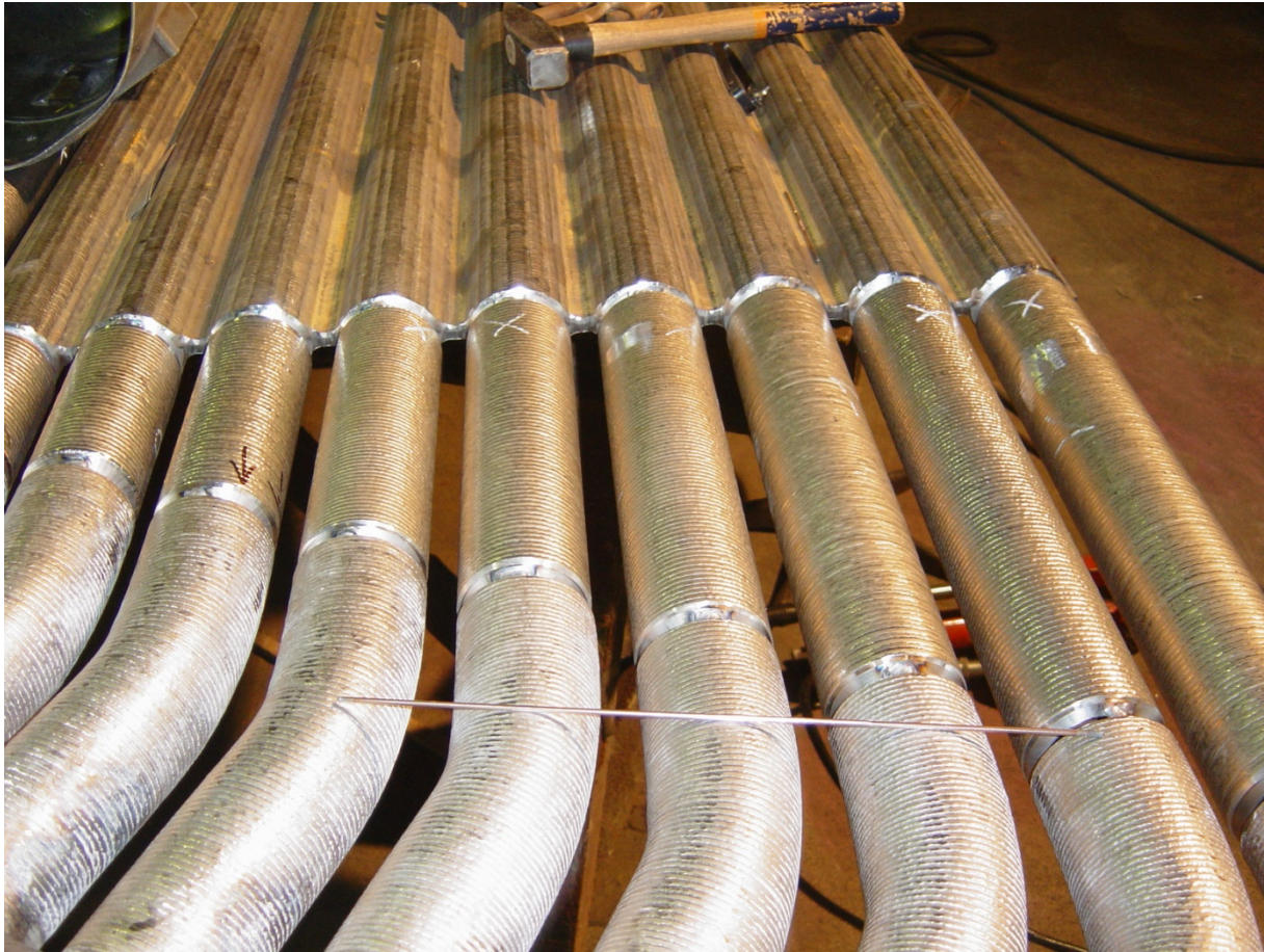
White / white connection of clad components
