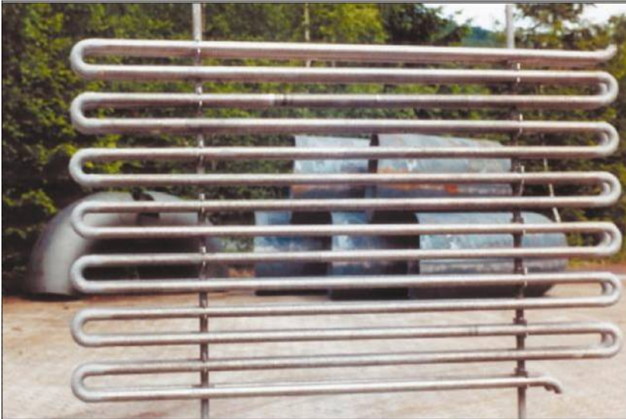
Cladded superheater tubes
