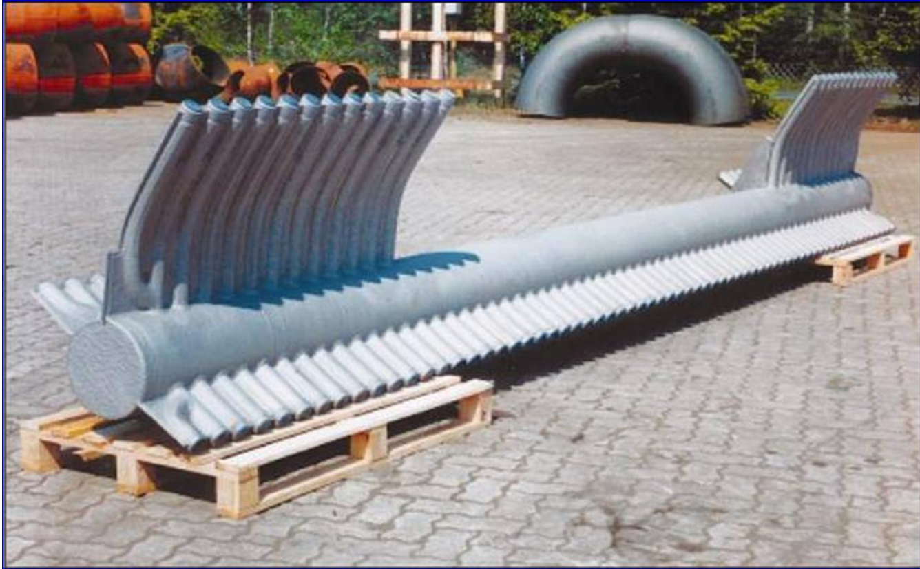
Cladded header with cladded, bended panel elements
