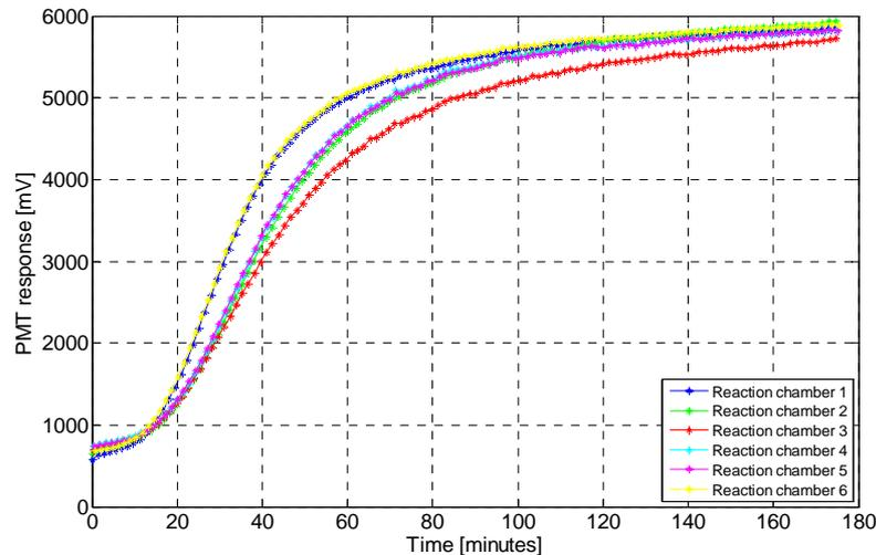
Figure 8. Amplification curves of the six 500 nl reaction chambers run simultaneously on one microchip employing a sample of positive control for HPV type 16 ( $0.1 \mu\text{M}$ ). The dried enzymes including PEG 8000 were re-hydrated after 1 day at room temperature. No amplification was observed when PEG 8000 was excluded in the drying procedure.
