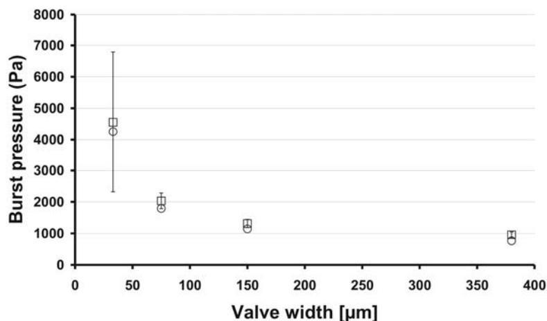
Figure 6. Burst pressures of the capillary valves as function of valve width. Symbols: □ DI water; ○ reagents; solid line represents the analytical values for water. Contact angle of DI water on Teflon was measured to be approx. 100°. The pressure data for each valve represents an average of 35 measurements (5 chips with 7 parallel channels each).
