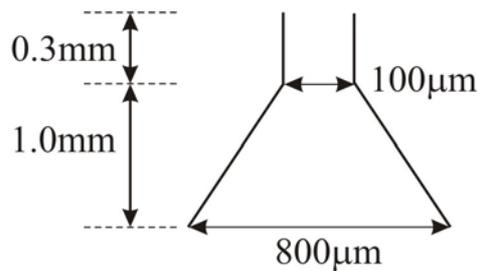
Figure 2. Details of capillary valve geometry (here, valve width is  $100\ \mu\text{m}$ ). The capillary valves contain a tapered part and a narrow restriction. The tapered part is included to aid spotting of the fluoropolymer for hydrophobization.
