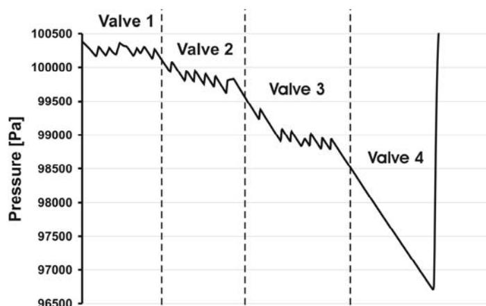
Figure 5. Common pulling pressure of parallel valves as a function of time. Parallel droplets are pulled at constant rate of 10  $\mu\text{l}/\text{min}$ . Absolute pressure trace of seven parallel droplets moving through the parallel actuation chip. At the fourth valve, the first droplet to break the valve effectively ventilates the system, and hence the pressure in the system returns to atmospheric conditions.
