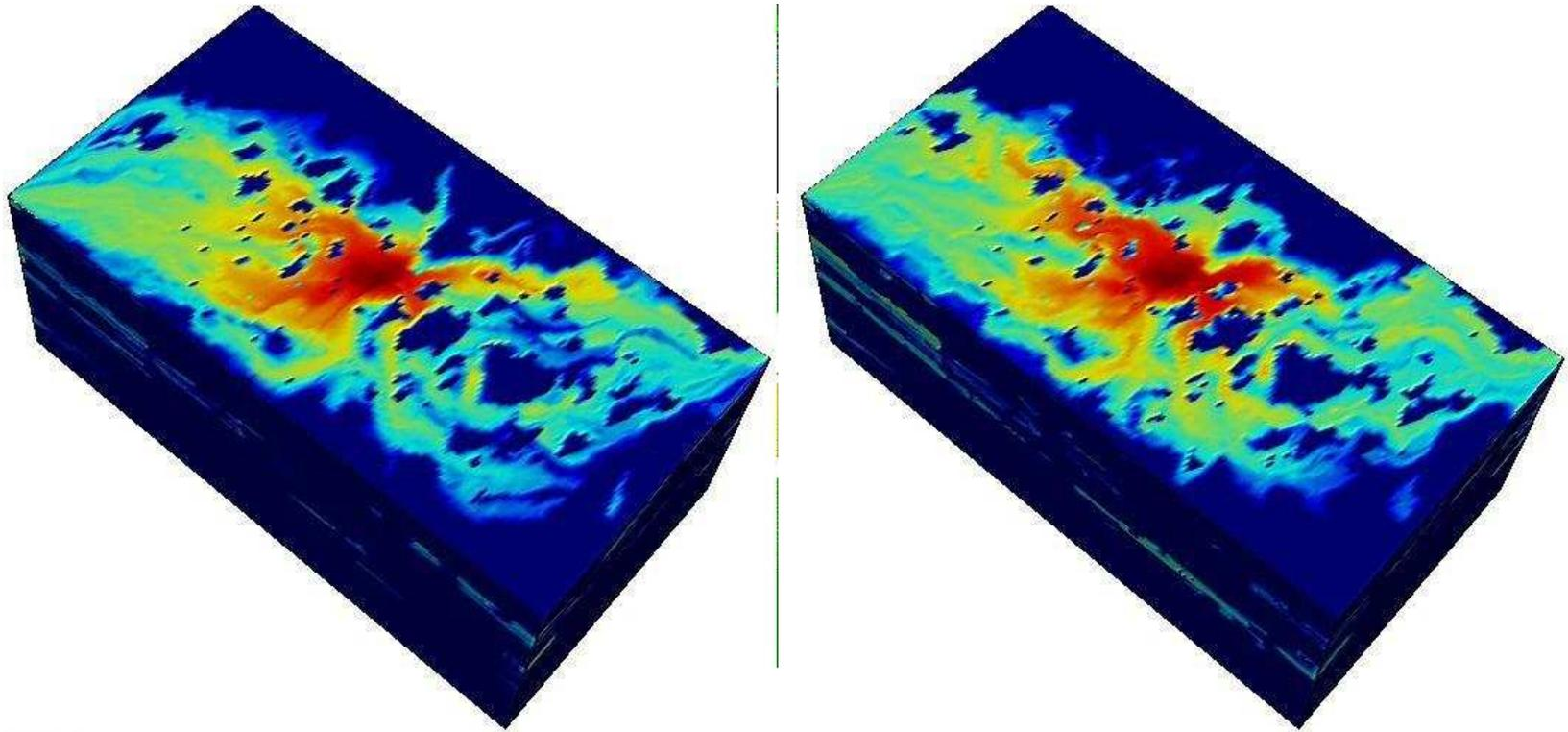
Our fine grid solution (left) and MMsFEM/Streamline solution (right) after 800 days of simulation.
