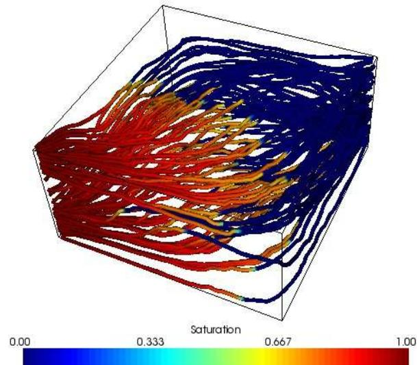
Saturations are moved forward along the streamlines under the assumption that the streamlines remain fixed during the time step.
