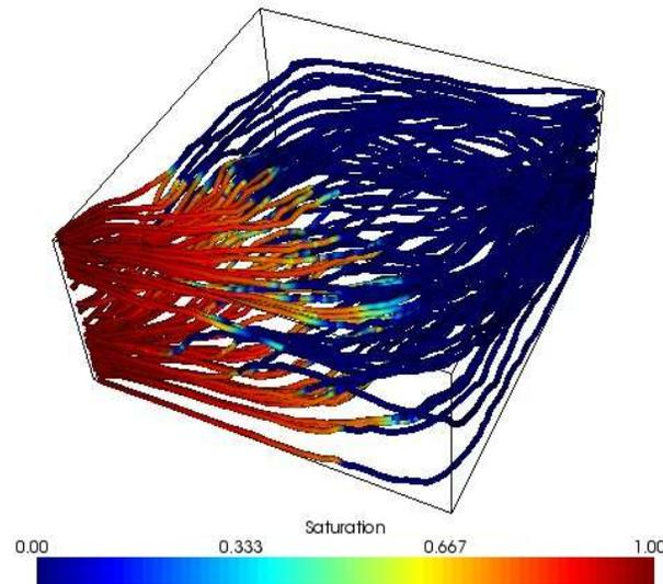
The pressure defines a velocity field and the streamline are traced from injectors to producers while picking up the grid block saturations.
