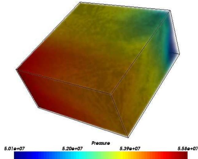
The pressure is computed using the initial saturations to evaluate the mobility terms.
