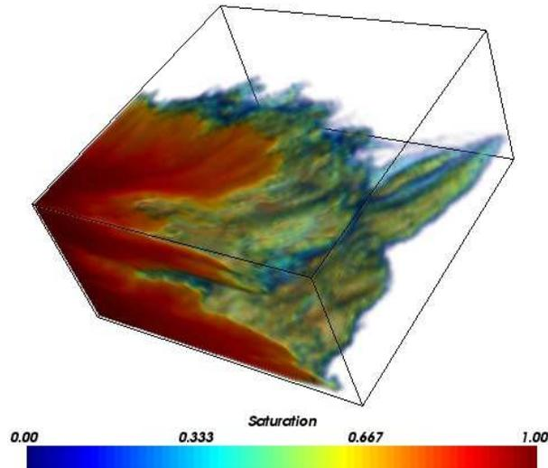
Finally the streamline saturations are mapped back onto the grid to yield a new saturation field, and the process may now be repeated.
