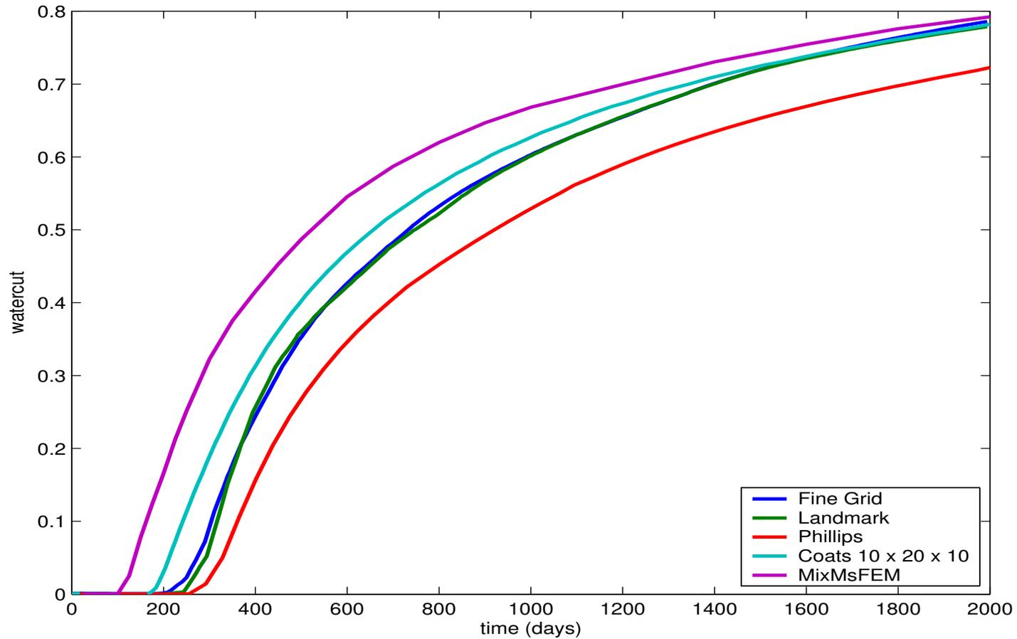
Water-cut curves comparing MMsFEM with various upscaled solutions.
