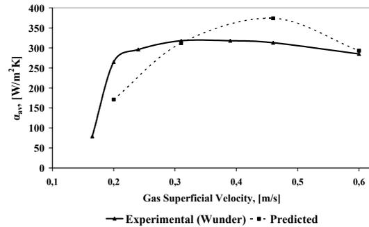
**Fig. 5** Effect of gas velocity on wall to bed heat transfer coefficient.
