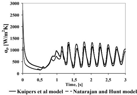
**Fig. 4a** Comparison between two solid phase thermal conductivity models.
