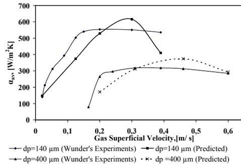
**Fig. 6** Effect of particle size on wall to bed heat transfer coefficient.
