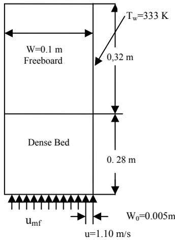
**Fig .1 Outline of a typical numerical setup.**
