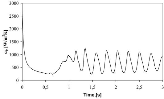
**Fig. 3b** Instantaneous heat transfer coefficient at a height of 0.15 m above the distributor.
