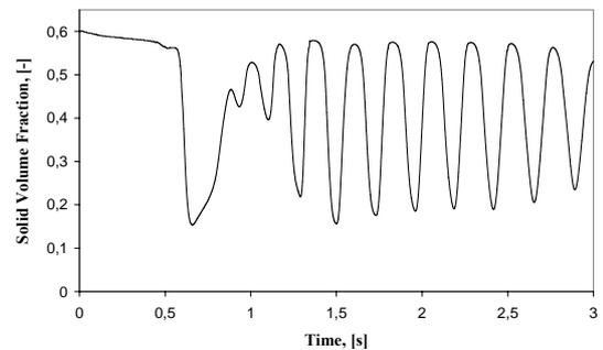
**Fig. 3a Temporal variation of solid volume fraction at a height of 0.15 m above the distributor.**
