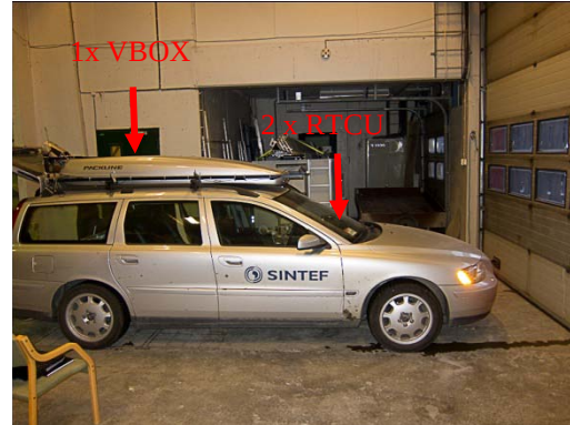
Figure 2 Placement of antennas on test vehicle
