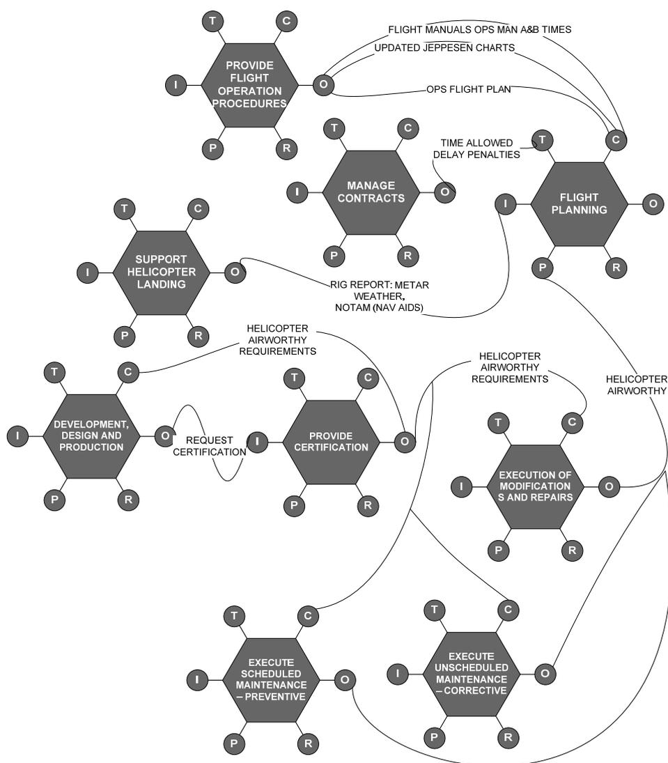
**Figure 9.2.** Selected elements of FRAM for scenario landing on helideck.
