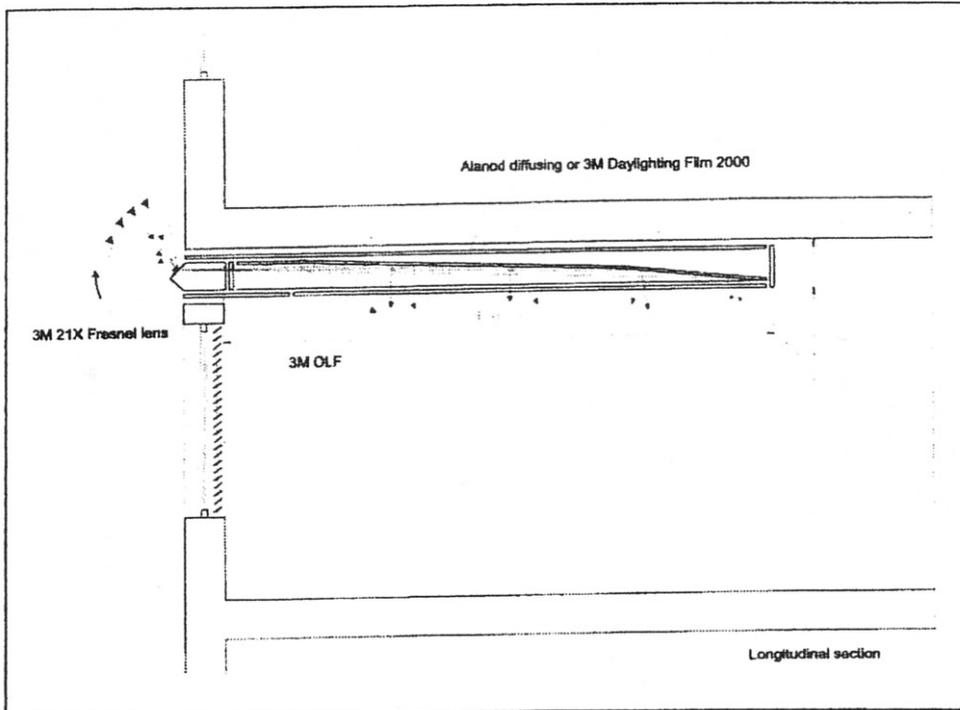
Figure 3. The Iguzzini hybrid lighting device.
