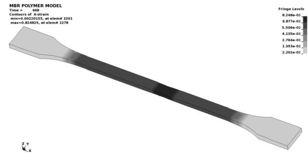
Figure 16 Strain localization prediction by introducing a geometrical imperfection.
