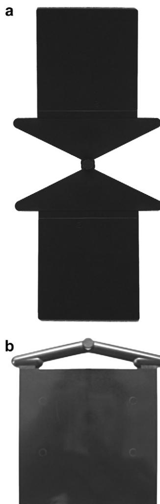
**Fig. 1.** (a) Injection-moulded plates ( $60 \times 60\text{ mm}^2$ ) with fan gates produced in a two-cavity mould, and (b) a plate ( $80 \times 80\text{ mm}^2$ ) filled from two adjacent corners, resulting in a weld line where the flow fronts from the two gates meet.
