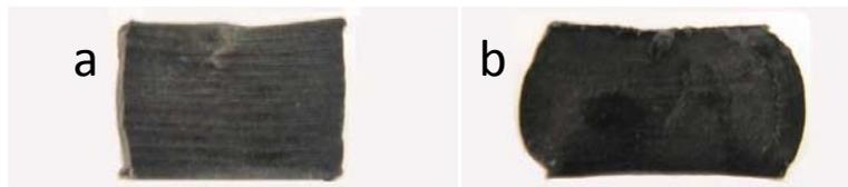
Figure 17 Barreling behaviour of lubricated test specimens with original dimensions  $4 \times 4 \times 4 \text{ mm}^3$  for a nominal strain of 50% (pictures after unloading). The specimens were machined from a dogbone (a) and a plate (b), respectively. In the pictures, the compression loading is vertical (and along the flow direction of the injection-moulded parts), and the as-moulded surfaces are vertical and into the paper plane.
