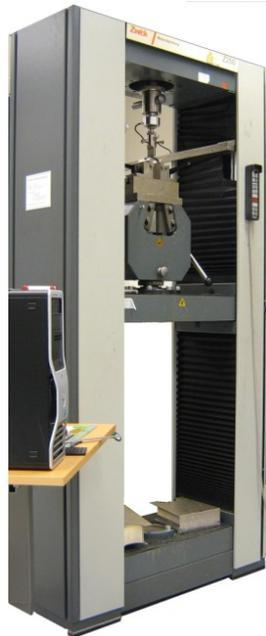
Figure 16 Zwick Z250 electromechanical universal testing machine at SINTEF
