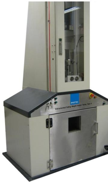
Figure 19 The instrumented falling-weight impact tester used in this thesis (Rosand type 4, modified by Imatek).
