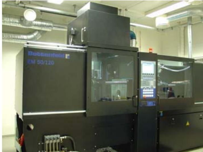
Figure 12 SINTEF's injection moulding machine. Battenfeld EM 50/120.
