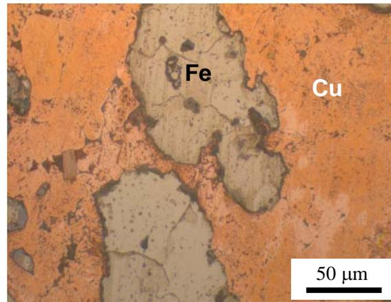
Figure 9. Iron powder particles in copper matrix.
