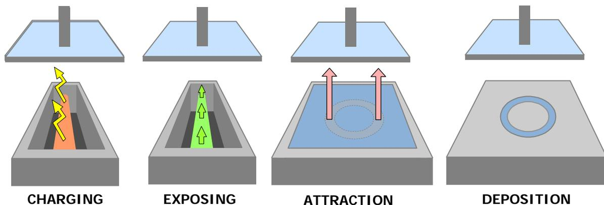
Figure 1. A schematic illustration of the process steps during layer fabrication.
