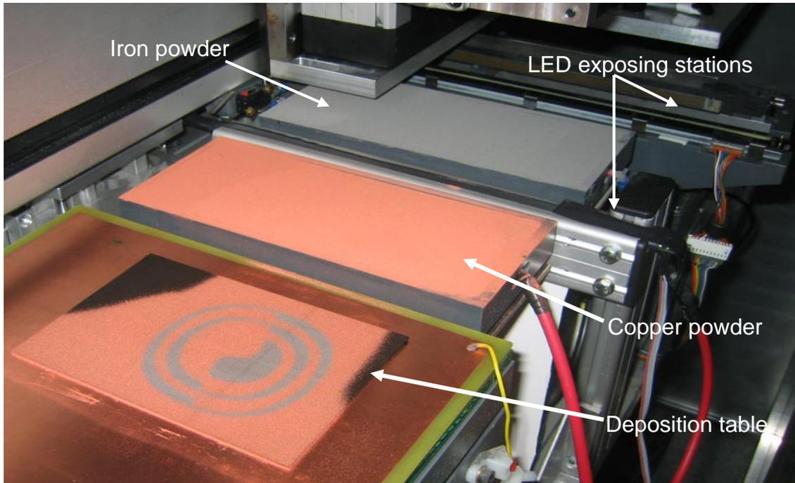
Figure 3. Layer fabrication of two different powders in the same layer.
