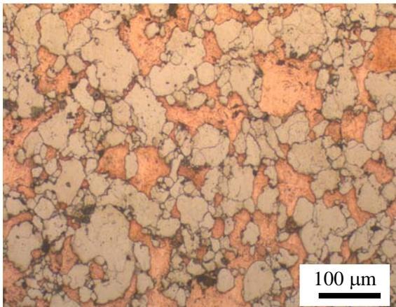
Figure 8. Distribution of Fe particles in Cu matrix.
