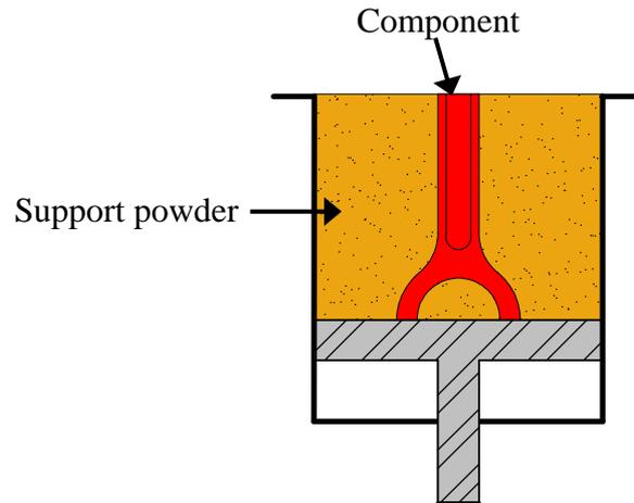
Figure 6. Method with which shaped components can be build using two different powders.
