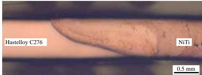
Fig. 6. Optical Micrograph of the NiTi-Hastelloy weld
