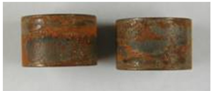
Oxidized and worn surfaces in erosion-corrosion
