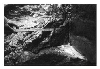
erwise a rapid destruction of the carbon blocks in the bottom and sidewalls of the electrolysis cells may be observed.
