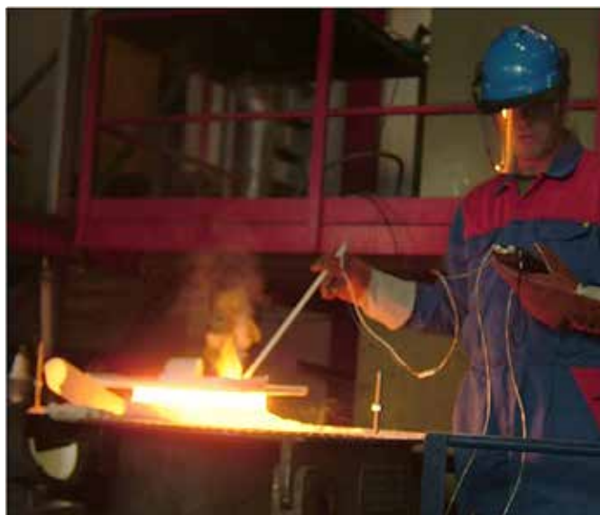
Temperature measurement during silicon refinement
