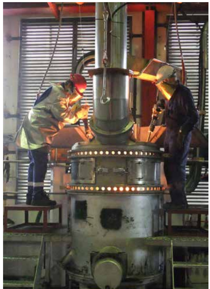
Production of silicon in the pilot scale reduction furnace at SINTEF
