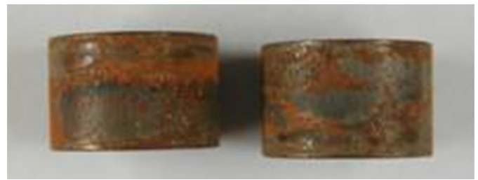
Oxidized and worn surfaces in erosion-corrosion samples
