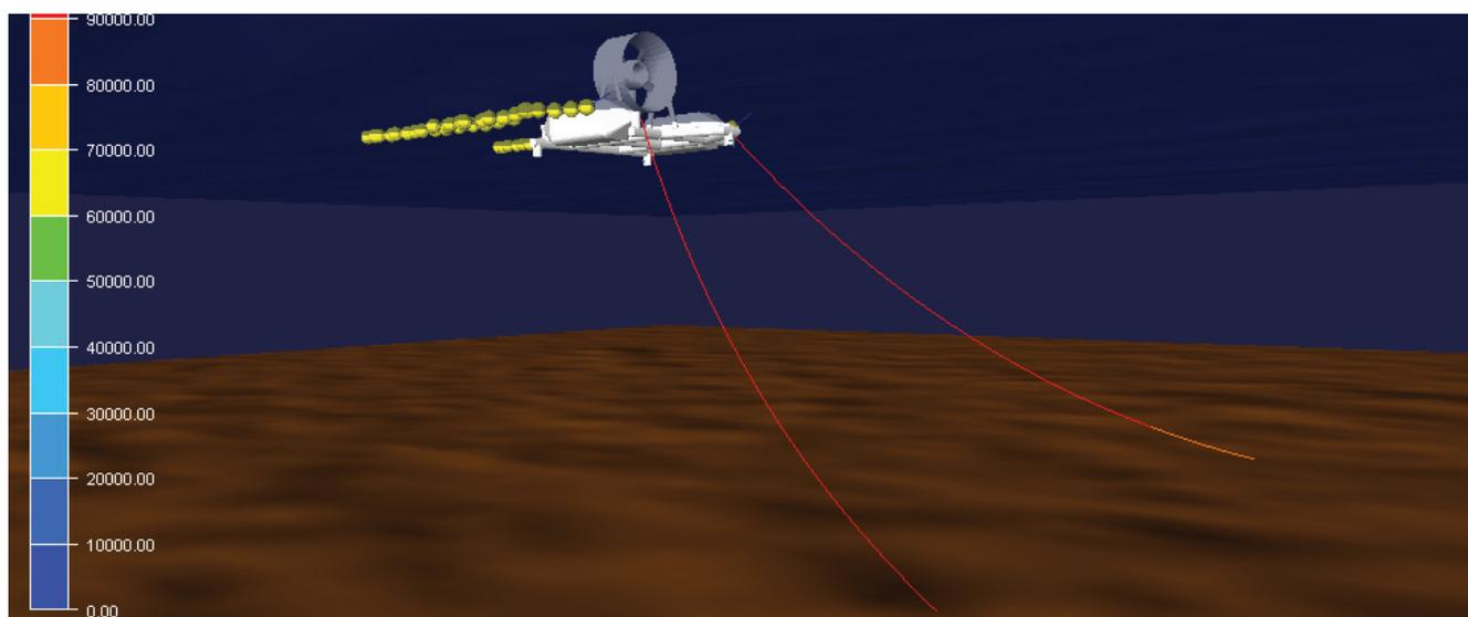
Figure 3. SIMO model of the system, unit on the surface (MARINTEK).
