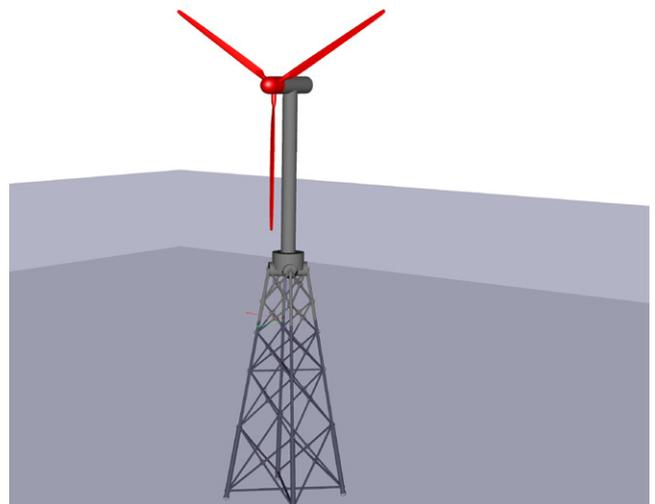
Figure 2. Simulation model of a Jacket type offshore wind turbine.
