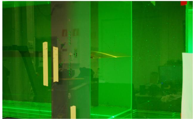
Figure 4. A wing model mounted wall-to-wall. The measurement plane is vertically orientated in mid-span position.
