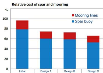
Figure 3. Examples of relative cost of spar buoy and mooring lines.
