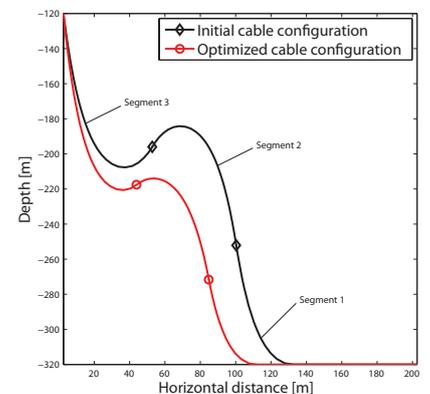
Figure 4. Example of optimization of power cable configuration.
