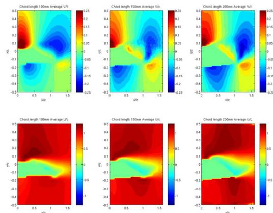
Figure 5. Results of the horizontal and vertical velocity component from three different model scales.
