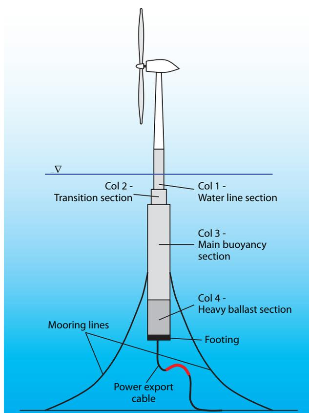
Figure 1. Wind turbine on a floating support structure. Idealization of spar buoy geometry.
