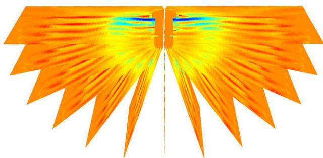
Figure 2. Visualization of the 13 different angular positions of the rotor relative to the PIV plane.
