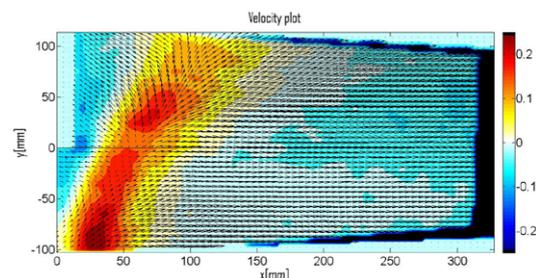
Figure 6. Time-averaged velocity field in the wake, revealing a spanwise flow from the smaller diameter end (below  $y=0$ ) to the larger diameter end (above  $y=0$ ).
