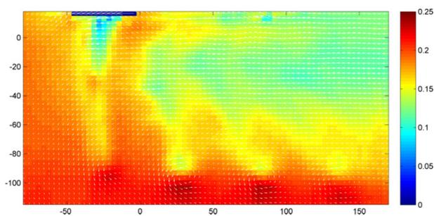
Figure 3. An example result of the time-averaged velocity magnitude reveals the defect downstream of the blade.
