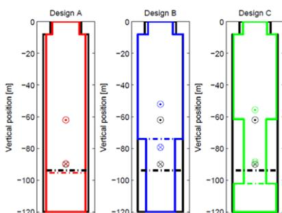
Figure 2. Examples of three different optimized designs of the spar buoy shape.
