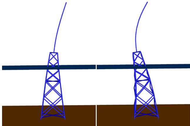
Figure 3. Modal analysis of the substructure global response.
