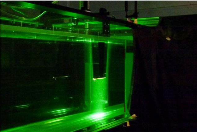
Figure 1. Tidal turbine model mounted inside the CWT lab. The flow is from left to right. A vertical plane is illuminated from below.
