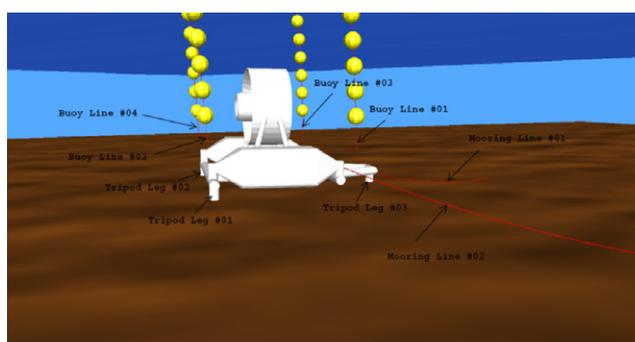
Figure 4. SIMO model of the system, unit landing on the seabed (MARINTEK).
