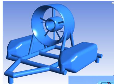
Figure 1. CAD model of the turbine. (Courtesy of Clean Current)
