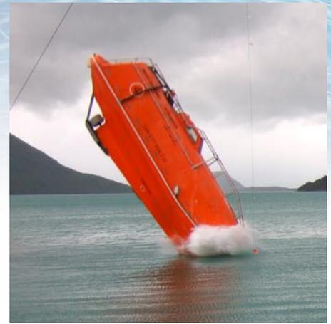
Figure 1. Full-scale testing of a free-fall lifeboat entering calm water.
