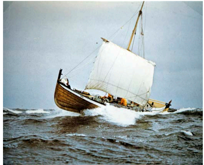
Fig.6. Traditional Norwegian (50ft.) square rig boat.
