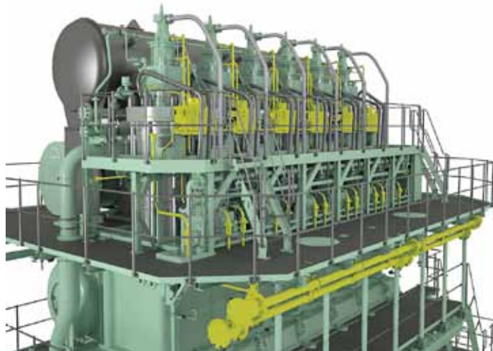
» Triality has two large two-stroke dual fuel main engines (MAN).
