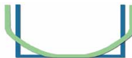
» Figure 3: Cross sections for Triality and a conventional VLCC
