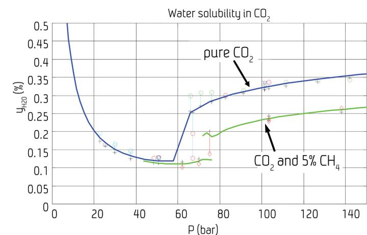
The impurities affect the thermodynamical properties of the CO<sub>2</sub> and thereby influence the compression, transport and injection process design and costs.
