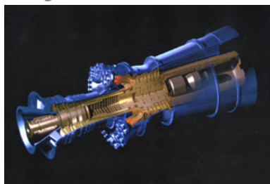
Cross-section of the GE MS9001H Advanced Gas Turbine Photo courtesy of DOE
