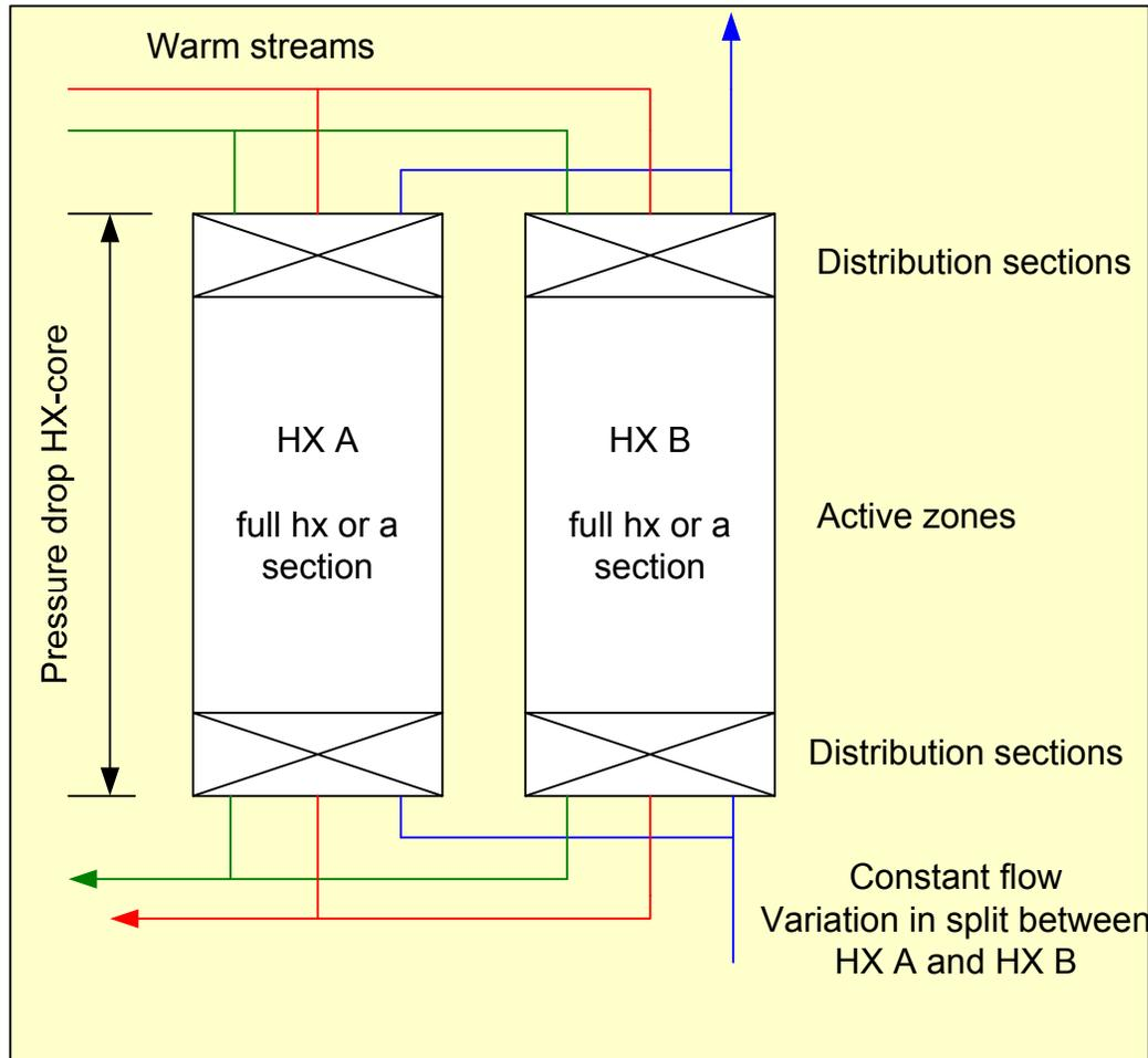
S-FIN can not simulate the Ledinegg instability conditions within one module
