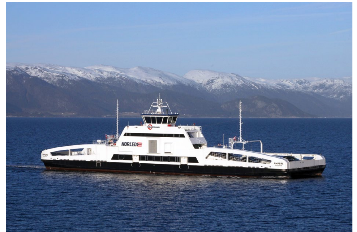
Figure 16: The world's first large electric car ferry, MF Ampere, launched 10 years ago by Norled (Source: Norled AS)
