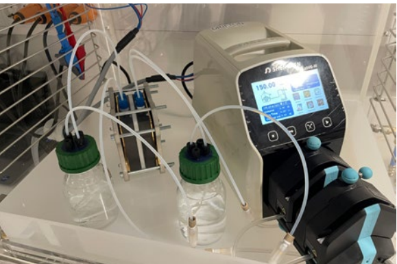
Figure 21: Flow battery test set-up for one flow battery cell (Photo: SINTEF).
