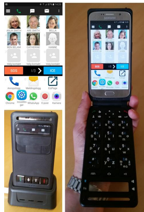
Figure 6 EziSmart Launcher user interface (upper left), Ezi-Pad with phone in charger crib (lower left) and Ezi-Pad with phone ready to use.
