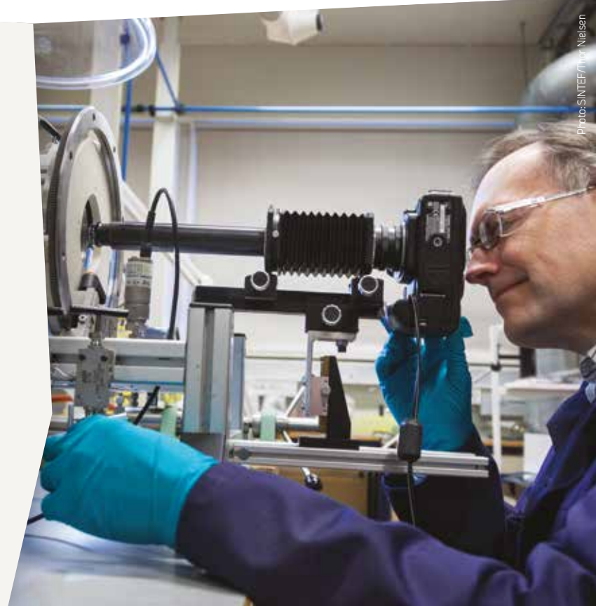
High pressure cell for measuring interfacial tension.
