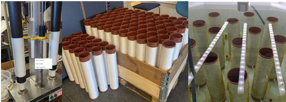
Fig. 2.1 Spools produced using a “spooling machine” (left and centre) at SINTEF Ocean and seeded by Seaweed Solutions (right).
