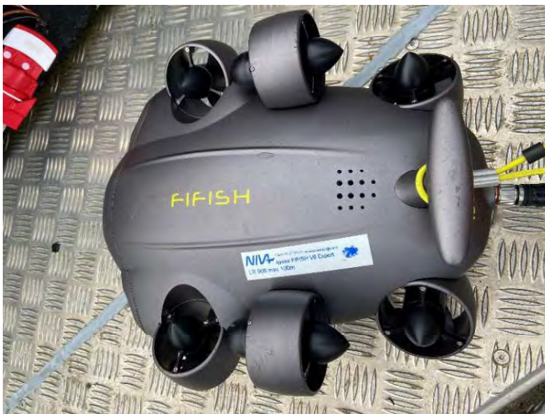
Figure 3. Ffish ROV used for sea floor mapping.
