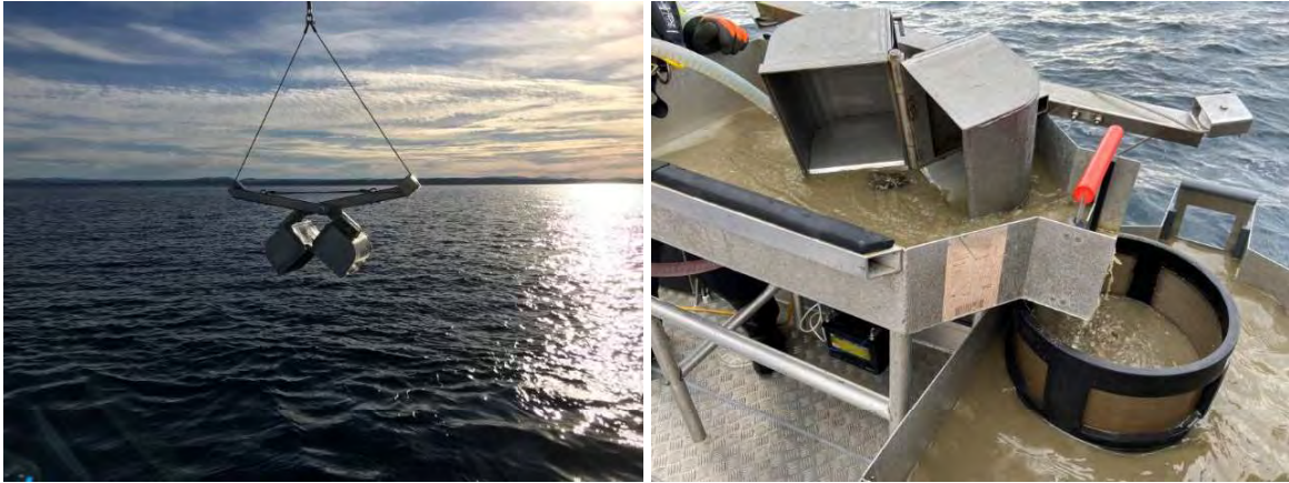
Figure 6 Field sampling of benthic fauna and sediment using a standard van Veen grab with a surface area of 0.1 m 2 and washing the material through sieves submerged in water for gentle treatment of the fragile animals.
