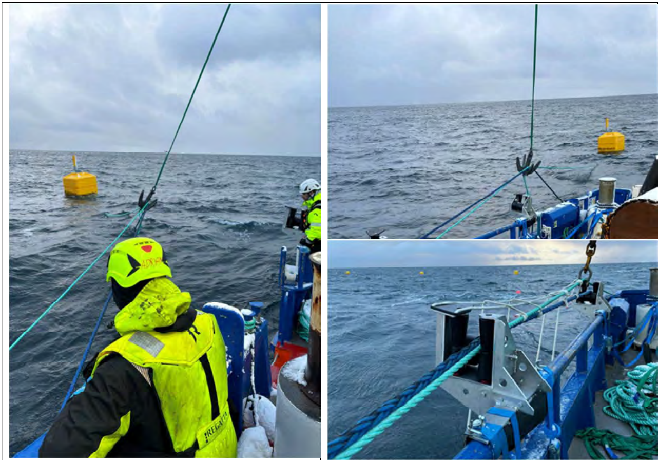
Figure 9: Lifting the mainline into the rope rollers
