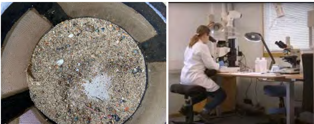
Figure 7 Left: sieve residue that was fixed with formaldehyde and brought back to the laboratory for sorting and species identification. Right: all individuals were identified to species level (if possible) and counted using a stereo microscope.
