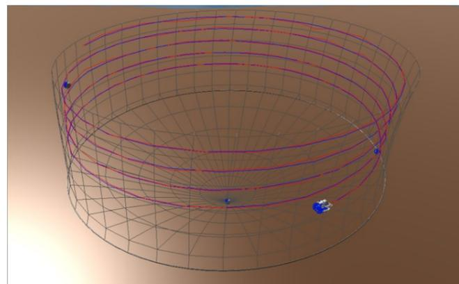
Figure 3: Autonomous navigation and net following.
