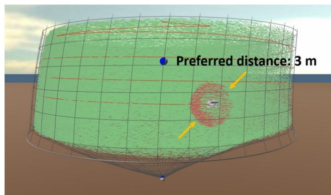
Figure 4 A: Simulation results for the fish behavioral responses toward ROV.
