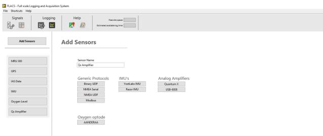
Generic protocols that are fully configurable on site are also implemented in FLACS. The protocols included are UDP Binary, UDP NMEA, Serial NMEA and Modbus. A variety of standard NMEA telegrams are described in FLACS and are automatically populated as they appear. Also for the binary data, FLACS has a list of predefined telegrams the operator can select from. There is no limit to how many instances of each sensor or generic protocols the user is allowed to add.
