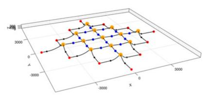
Modal wave and wind loads analyses, and extreme value statistics of key quantities for the wind park, such as relative and absolute offset between turbines, tensions in the shared and anchored lines. etc. Complete dynamic analysis of floating
