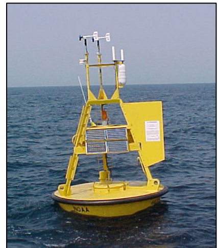
Figure 4 - National Data Buoy Centre operated 3-meter discus buoy for taking weather and marine observations (image from www.ndbc.noaa.gov )
