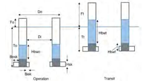
Figure 1: Illustration of the design variables of the floating dock
