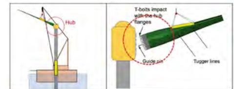
Figure 3: Blade root sideways impact and damage in guide pin and root laminate
