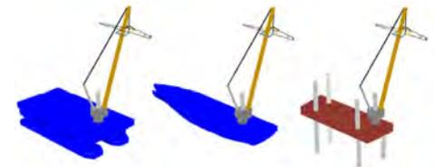
Figure 2: Illustration of single blade installation using semi-submersible, mono-hull and jack-up installation vessels
