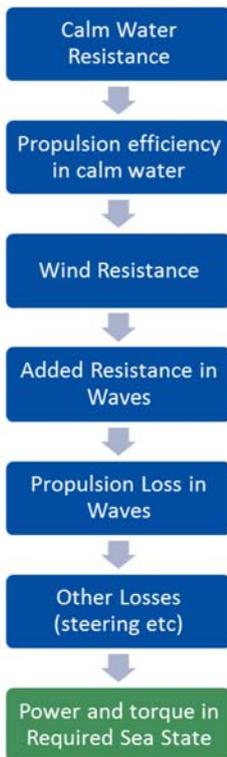
There are several calculation steps required to find the required power and torque to maintain 6 knots in a sea state.
