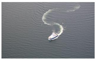
Test according to IMO's 2000 HSC Code and Annex 9 testing. Cruise performance in moderate and rough seas. Turning and manoeuvrability tests. Stopping and accelerations tests. Failure testing (FMEA-tests). Tests to document limiting of safe operation of the craft. – (Comfort, motion and acceleration. Operational criteria and limitations).
