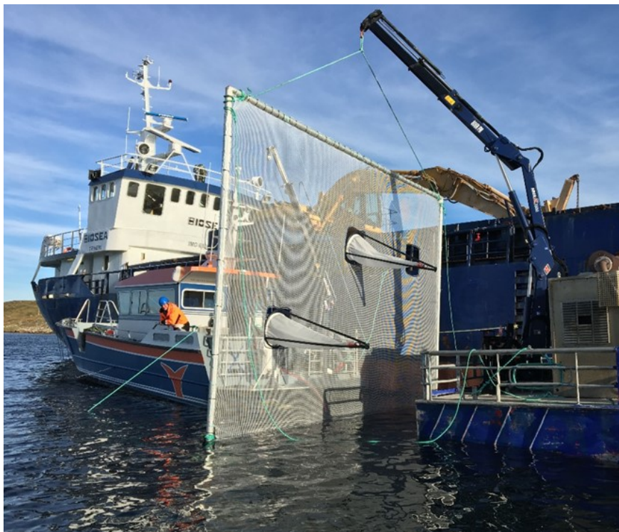
Figure 1: Setup for the conduction of net cleaning experiments where biofouling cleaning waste was collected.
