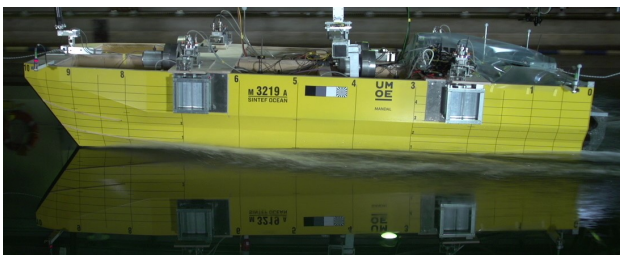
Figure 1: Surface Effect Ship as Crew Transfer Vessel for Oil and Gas Market. Courtesy of UMOE Mandal AS
