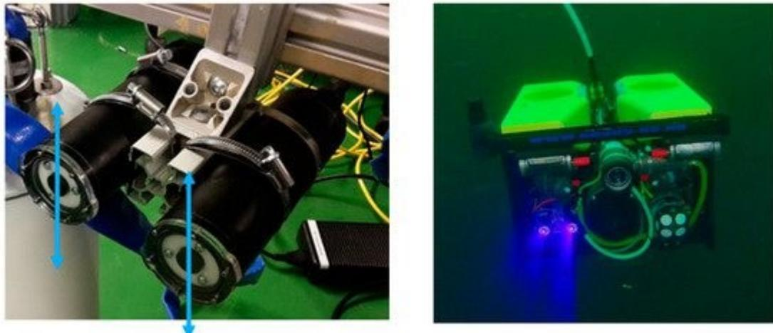
Figure 3. Left: The lasers are mounted inside watertight tubes. Photo courtesy of SINTEF Digital. Right: The lasers mounted onto the ROV. The camera used is the on-board ROV camera, seen in the center of the ROV. Photo courtesy of SINTEF Ocean
